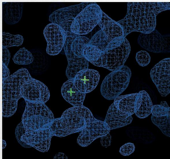
**Highly accurate data: EIGER detectors are capable of delivering outstanding data quality. Data were collected from an insulin crystal at 12 keV with an EIGER 1M prototype at a detector distance of 60 mm. Only 360° of data are sufficient for successful S-SAD phasing at 12 keV.**
